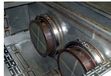
Inside view of Filter/Silencer Design using PERMIT™ FBC Filters
